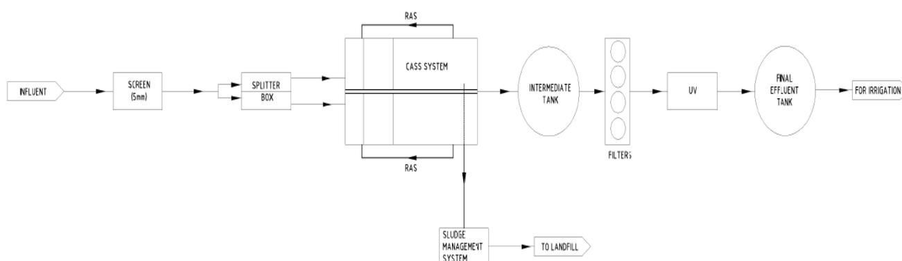
Figure 1: Basic Schematic Diagram of the Mangawhai WWTP.
