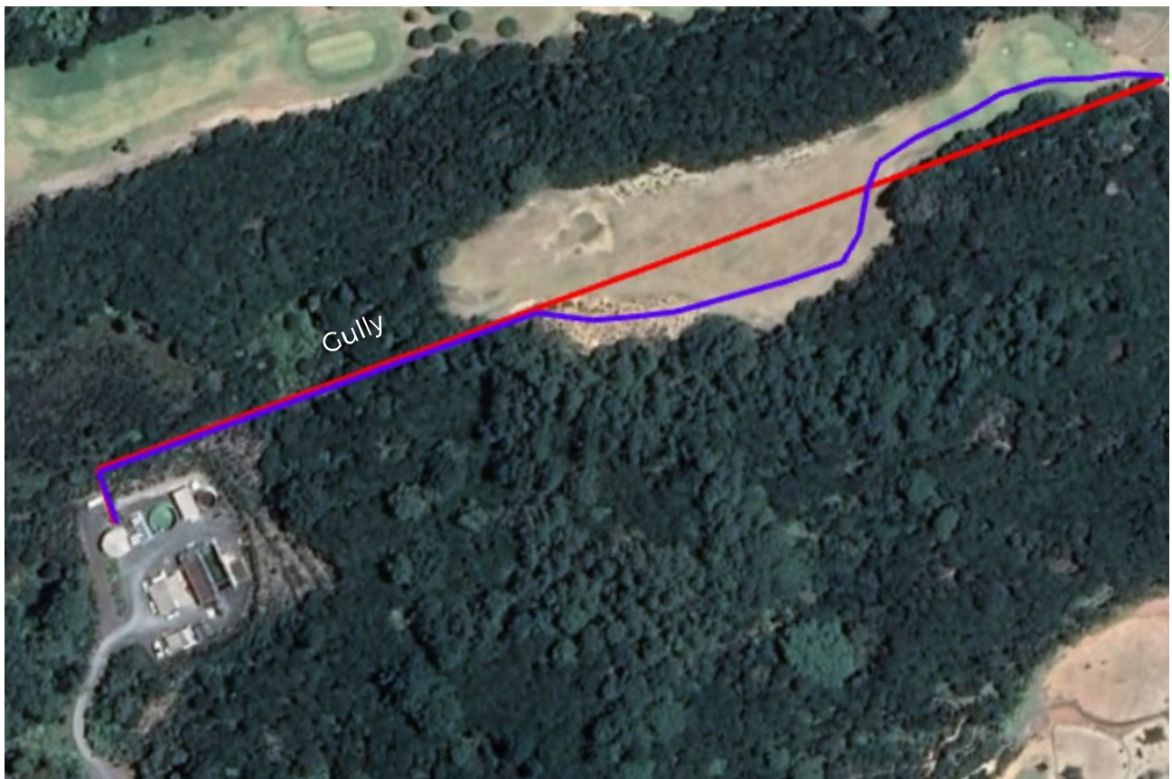
Figure 4, Pipeline routing options from WWTP to Location D. Red line indicates possible directional drilling route, and blue line possible trenching route.
