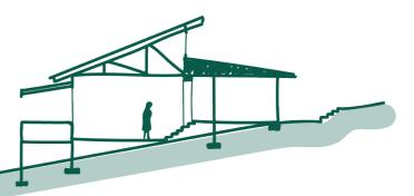
Stepped floor levels approximate 15% slope (south facing slope)
