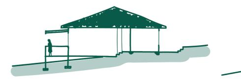
Stepped floor levels approximate 10% slope (north facing slope)
