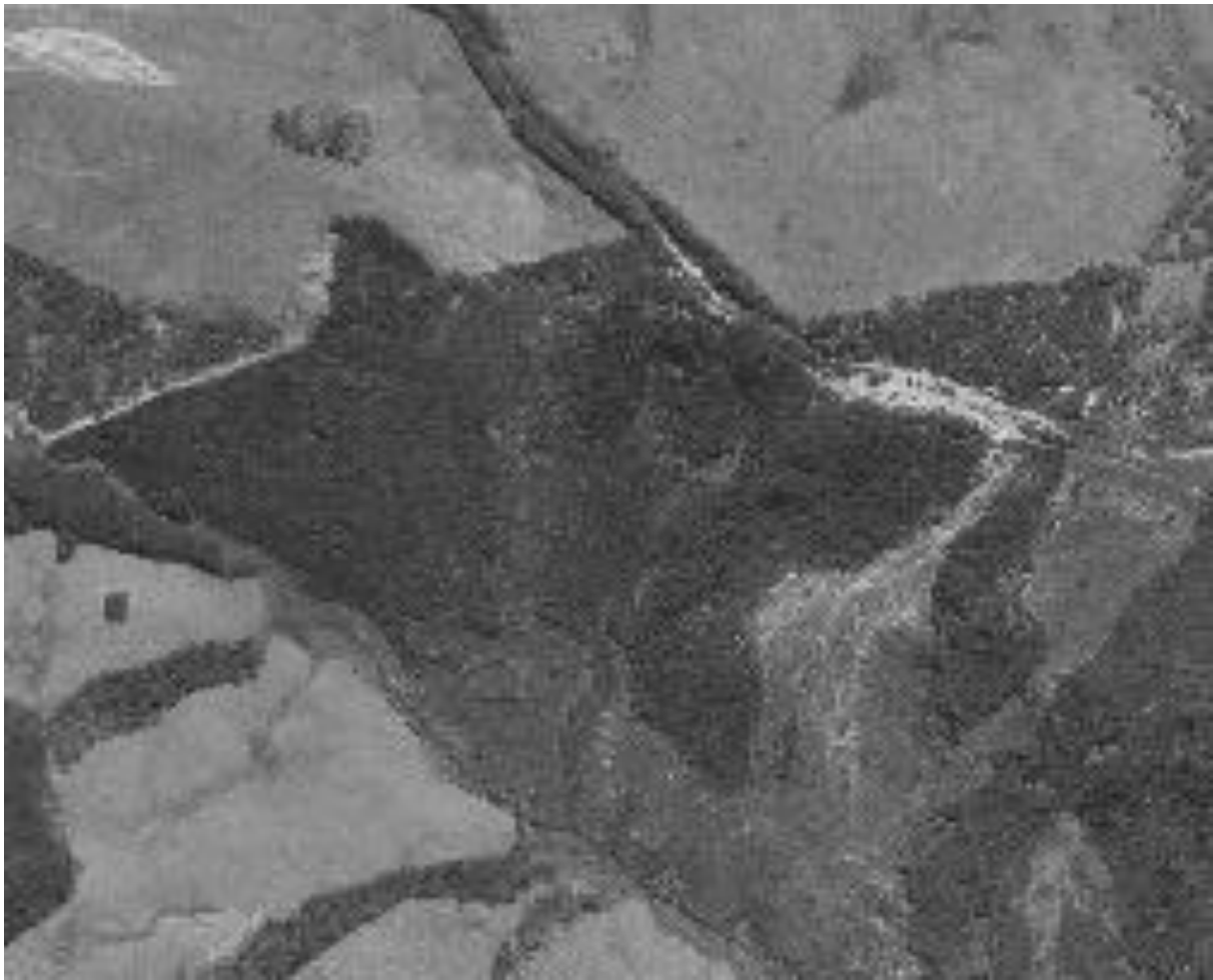
Figure 29: Detail from 1961 aerial showing scouring/erosion and vegetation on the two spurs.
