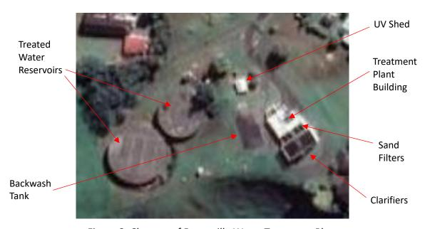
Figure 2: Close up of Dargaville Water Treatment Plant
