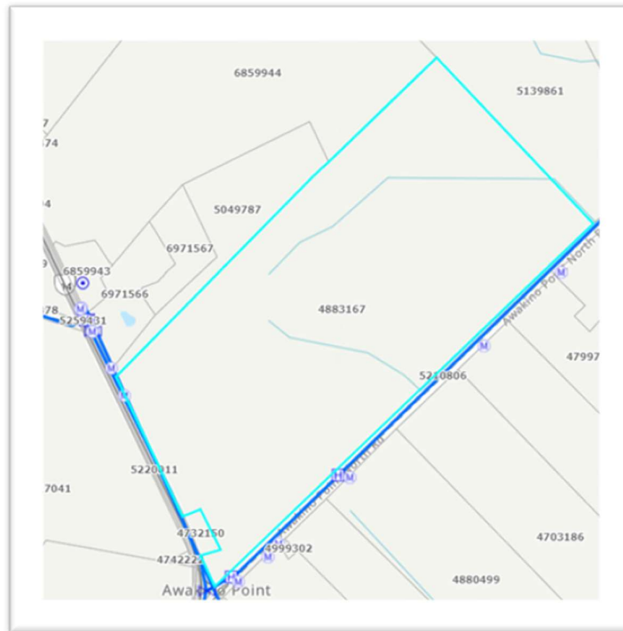
Figure 20: Map extract depicting 100mm and 180mm diameter water mains along the western and southern boundaries of the site (Source: KDC Utility Services Maps)
